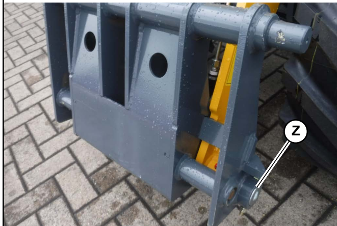
Fig. 116 – Attachment Locking Pins Retracted
