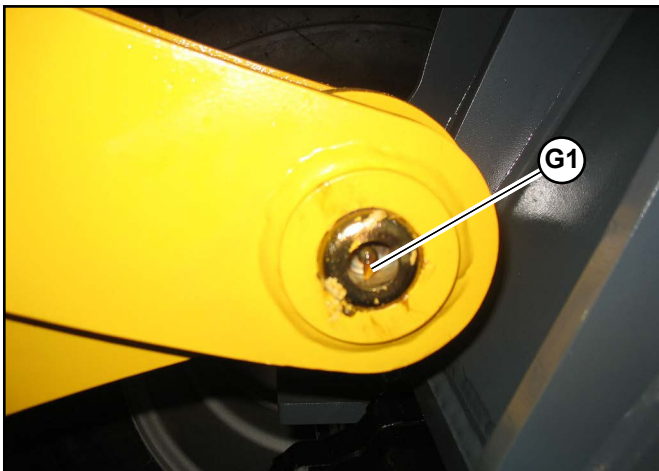
Fig. 162 – Lubrication - Non-Telescopic Machines - Bottom Tilt Link Pivot
