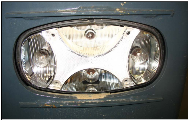
Fig. 239 – Left Tail Light Bulbs
