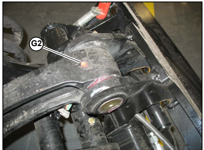
Fig. 171 – Lubrication - Telescopic Machines - Hitch Pivot Top
