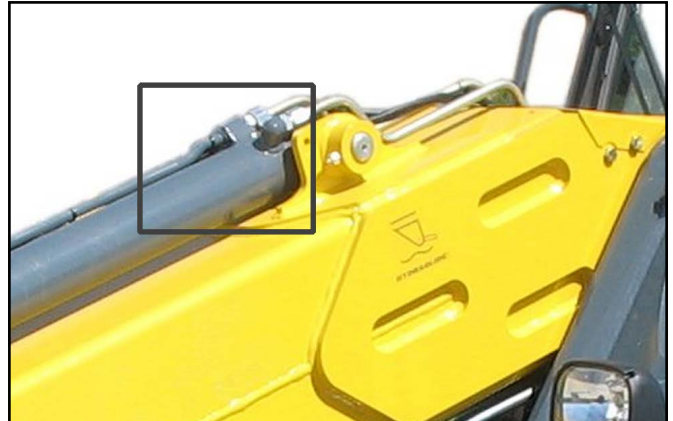
Fig. 2 – No Counterbalance Valve (Early Series Telescopic Machines)
