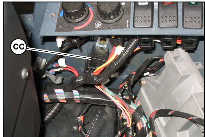
Fig. 232 – Front Wiper Relay (Inside HVAC Control Panel)
