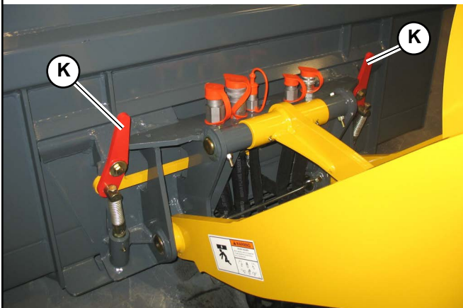
Fig. 111 – Attachment Hitch – Locked
