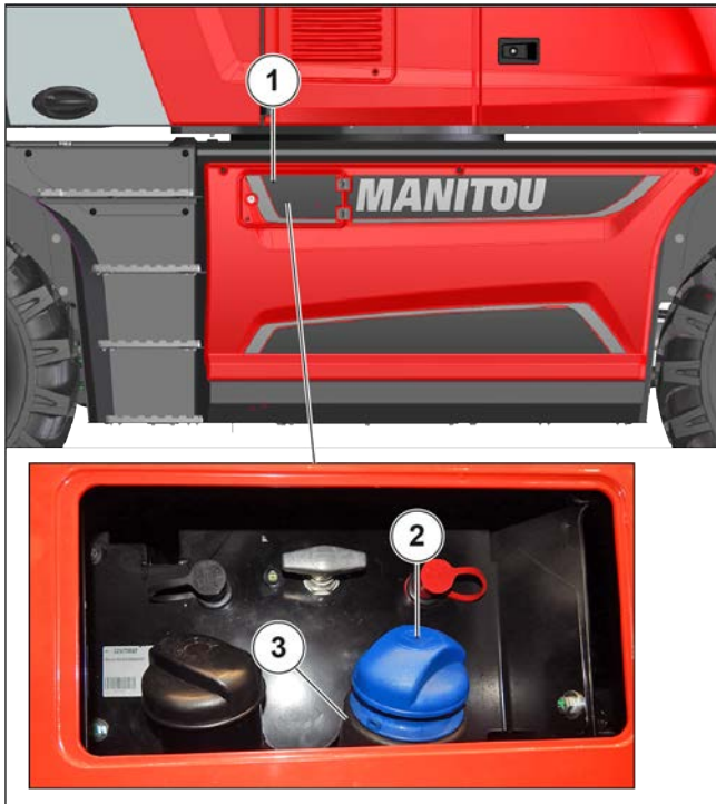
Figure 149: Checking DEF liquid level
