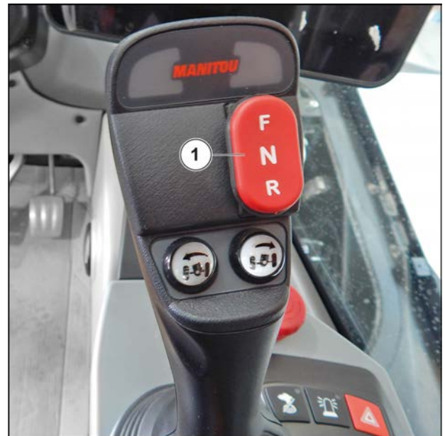
Figure 132: Using the FNR selector
