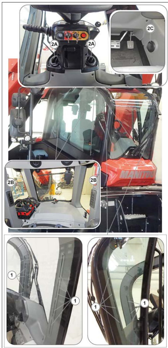
Figure 62: Demisting diffusers and heating air vents
