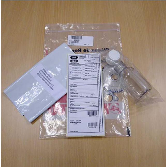
Figure 173: Hydraulic oil contamination check
