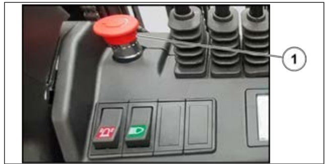
Figure 26: Emergency stop button
