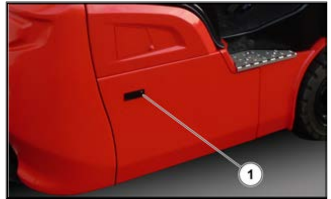
Figure 74: Battery tray side door
