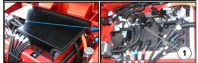
Figure 85: Check power fuses
