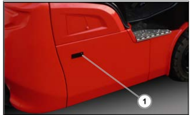
Figure 51: Battery tray side door
