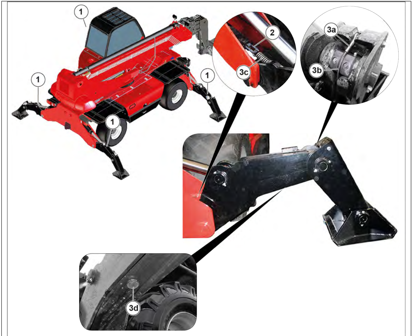
Figure 288: Replacing the internal stabilizer components
