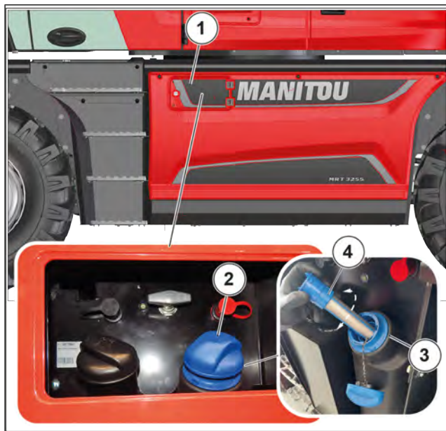
Figure 308: Checking and cleaning the DEF tank filler filter
