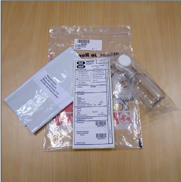
Figure 261: Hydraulic oil contamination check
