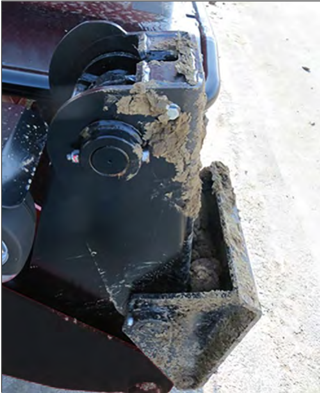
Figure 222: Removing debris and dirt from the stabilizers.
