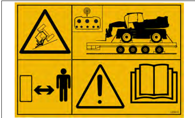
Figure 38: Decal - Warning Risk of rollover
