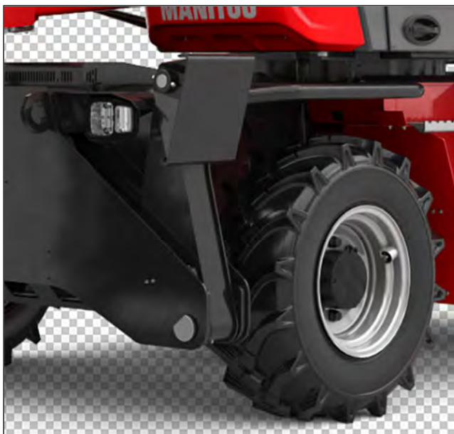
Figure 225: Road Traffic - Stabilizers completely closed (MRT 1645 - MRT 1845)
