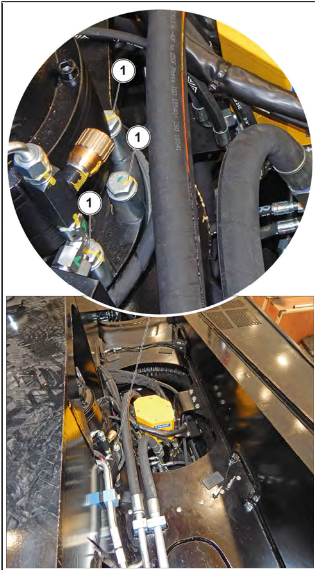
Figure 255: Rotation reducer fixing screw tightening check
