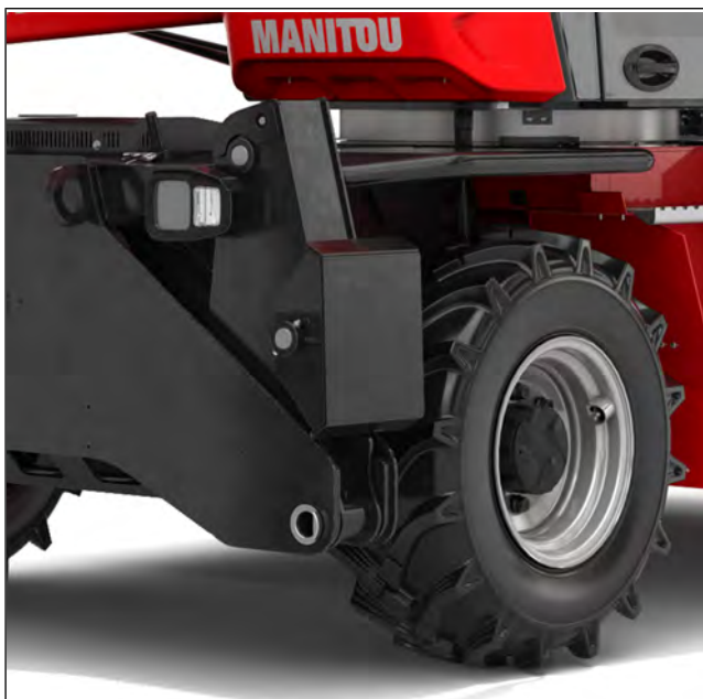
Figure 226: Road Traffic - Stabilizers completely closed (MRT 2145 - MRT 2545)
