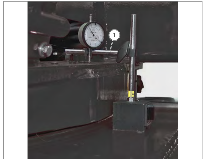
Figure 285: Check for wear and increase in clearance of the fifth wheel bearings
