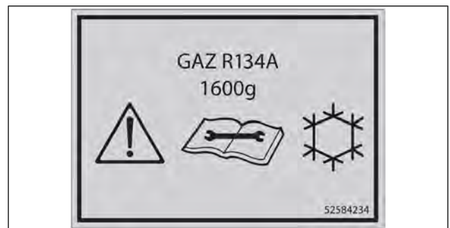
Figure 54: Recharge of air conditioning system
