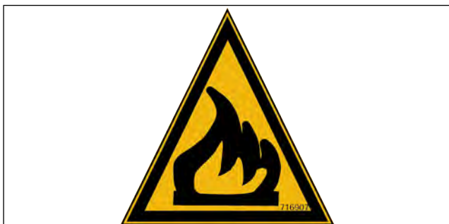
Figure 29: Decal - Danger Flammable liquids
