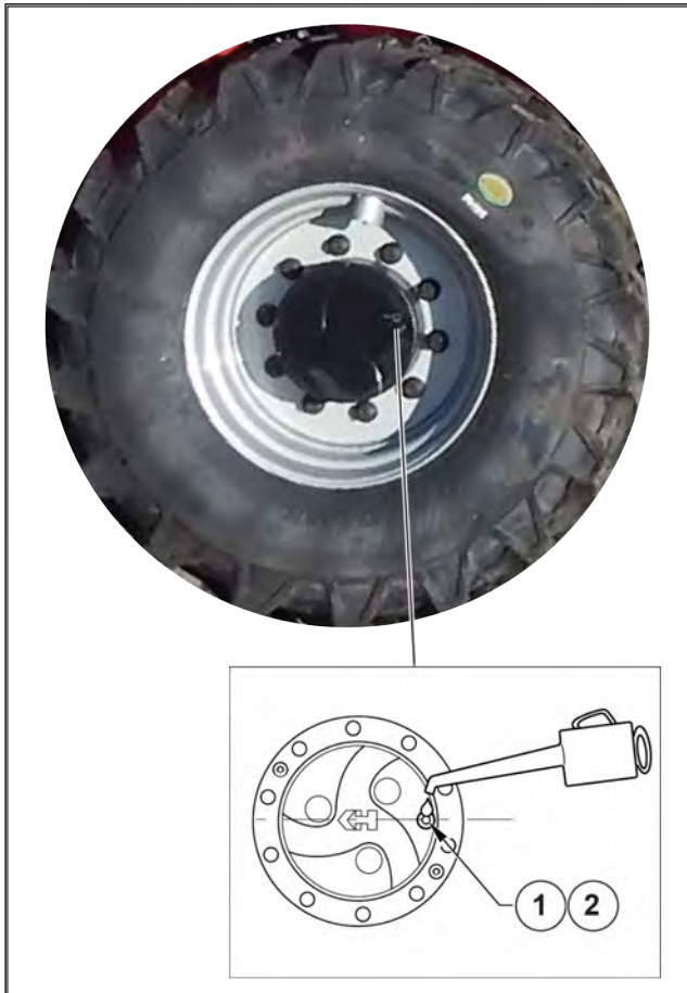
Figure 252: Front and rear wheel reducer oil level check
