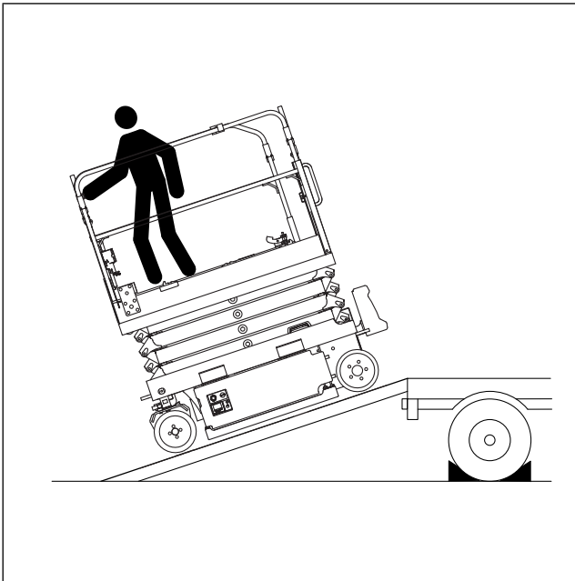
Figure 72: Unloading the machine on a transportation vehicle
