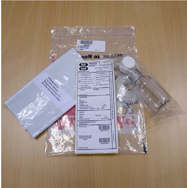
Figure 173: Hydraulic oil contamination check
