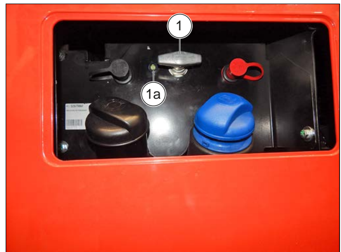
Figure 66: Battery disconnect switch
