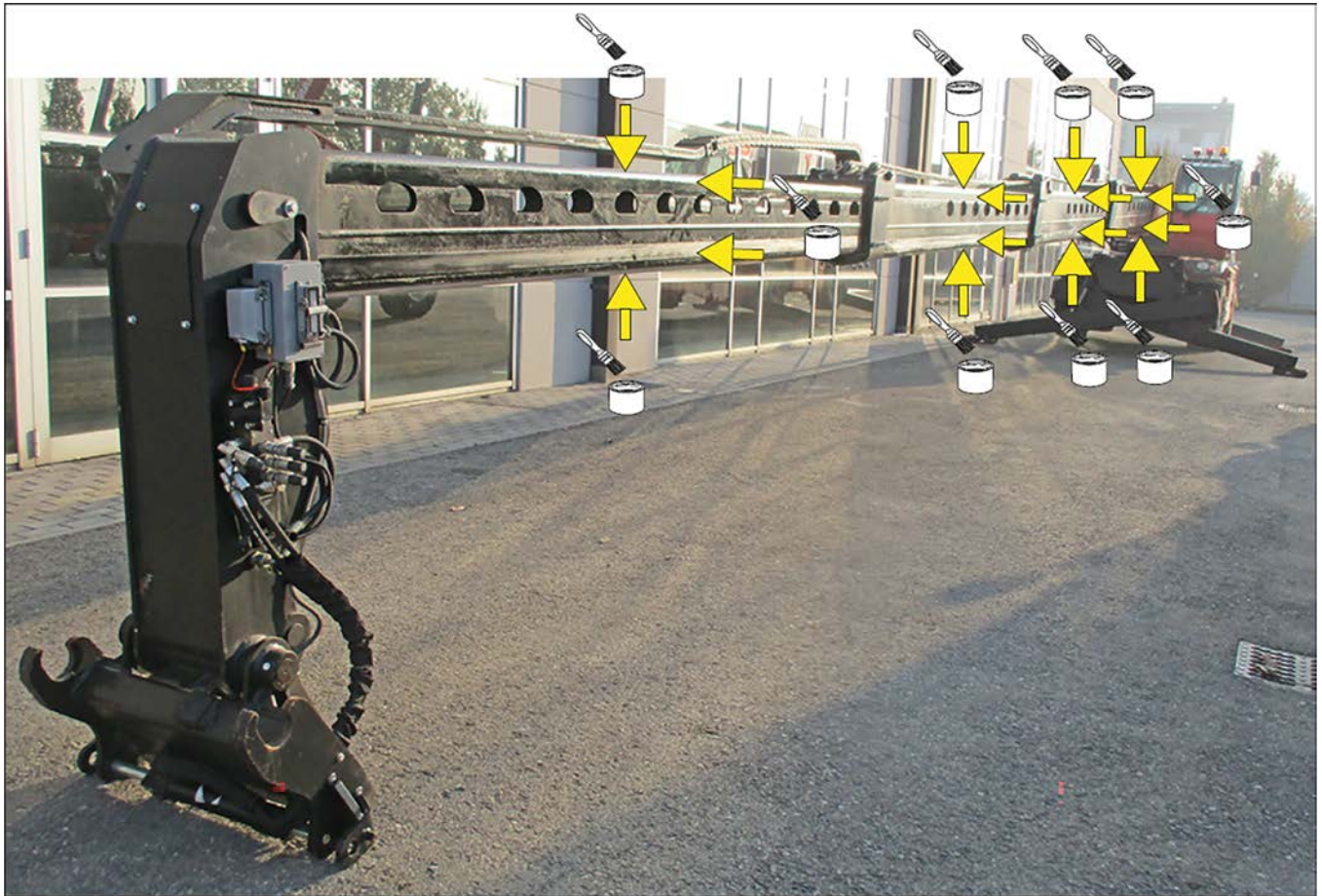
Figure 156: Cleaning and lubricating the telescopic boom wear shoes
