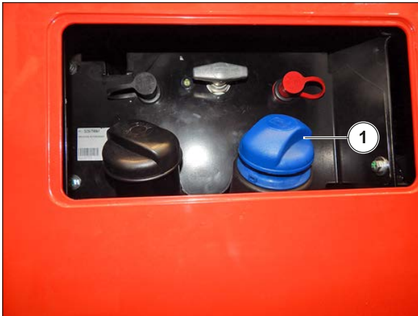
Figure 122: Filling the "DEF" tank
