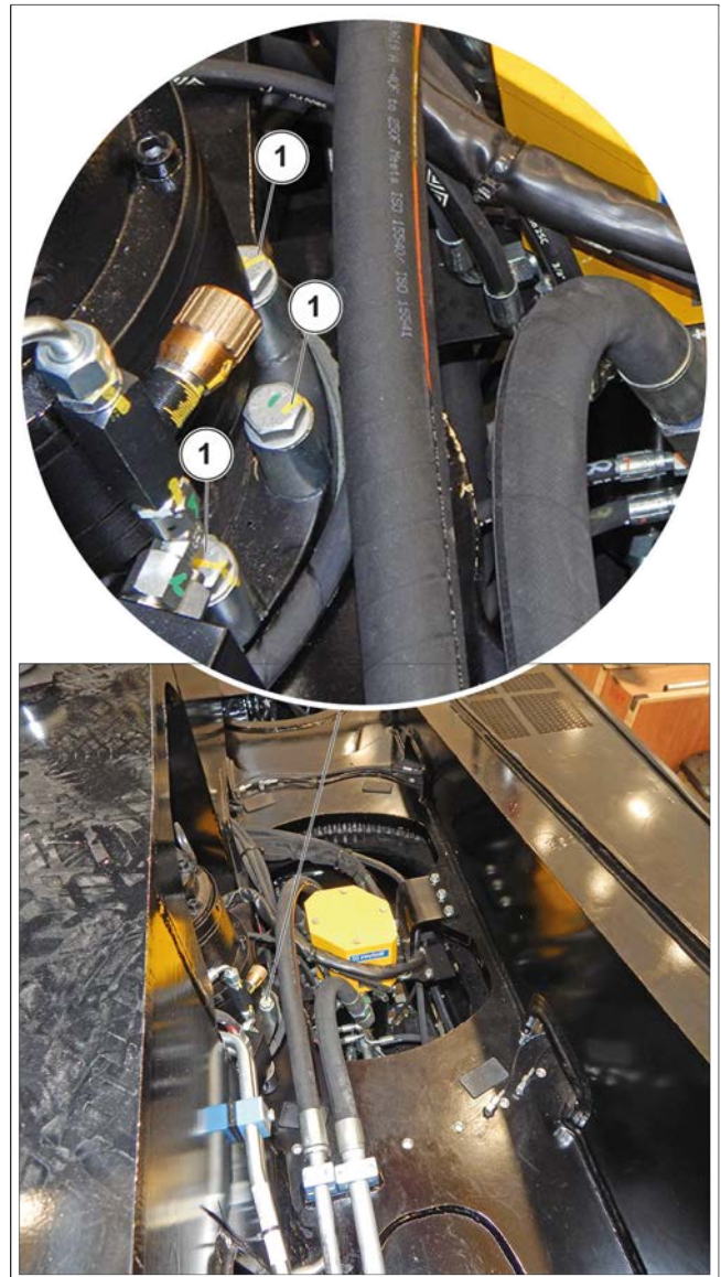
Figure 166: Rotation reducer fixing screw tightening check
