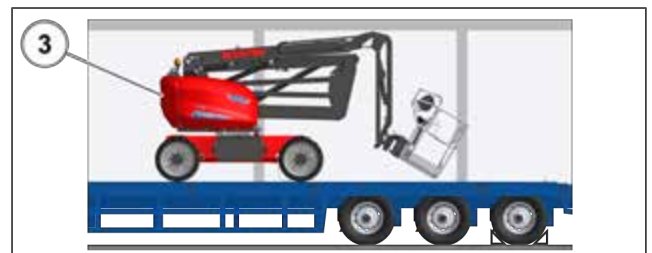
Figure 76: Machine in transport position (3)
