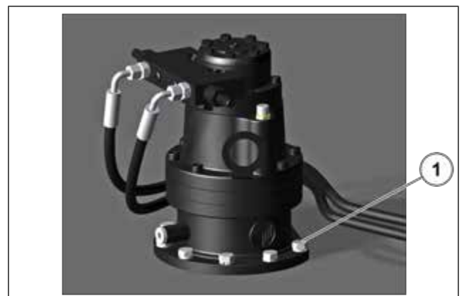
Figure 136: Checking the tightness of the turntable rotation motor
