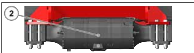
Figure 87: Checking the rear axle differential for leaks
