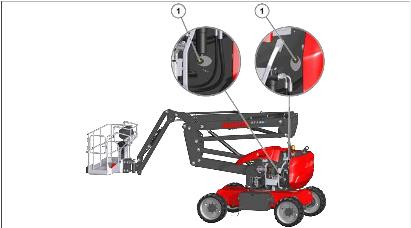
Figure 106: Lifting structure lubrication 4
