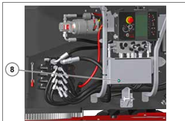
Figure 29: Electric centralized filling for high-voltage batteries 2
