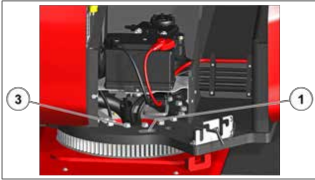
Figure 134: Checking the tightness of the crown gear assembly 1
