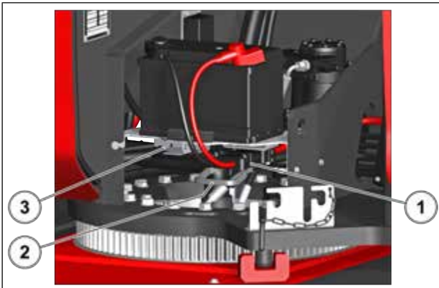
Figure 41: 12 V battery connector connected
