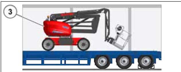
Figure 72: Machine in folded position (3)
