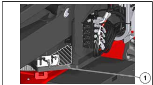
Figure 32: Tilt sensor calibration test
