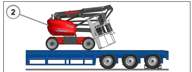
Figure 75: Machine in transport position (2)
