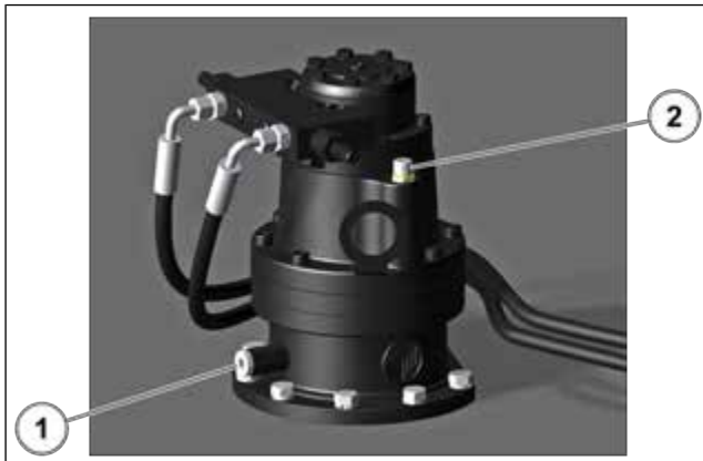
Figure 141: Replacement of the turntable rotation motor oil 1
