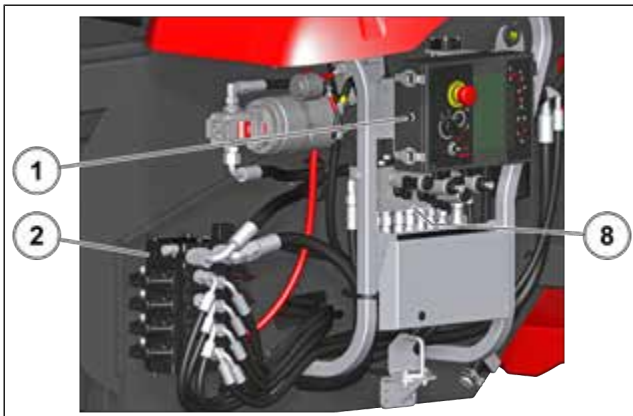
Figure 49: Location of the emergency controls 1
