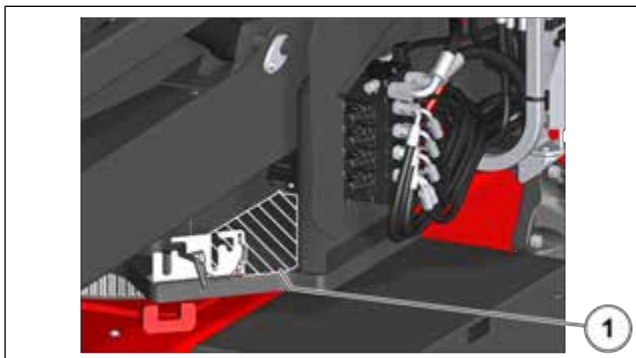
Figure 123: Checking the tilt sensor calibration
