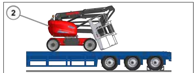
Figure 71: Machine in folded position (2)
