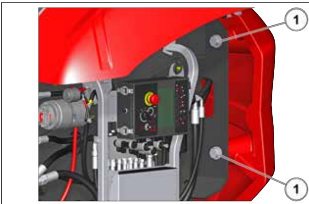
Figure 137: Checking counterweight 1 tightening torque
