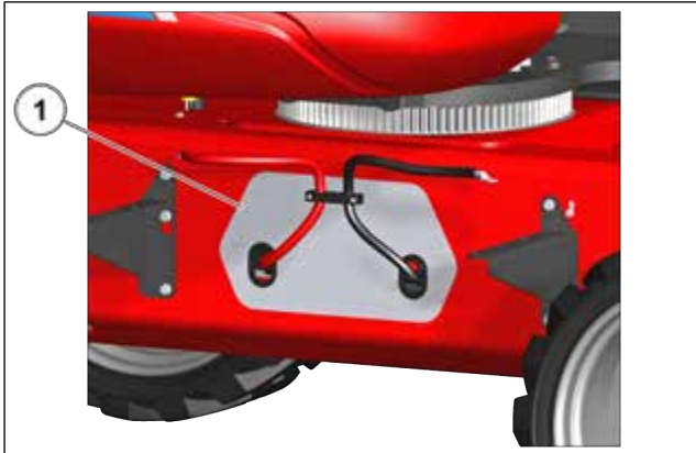
Figure 113: Checking the tightness of the high-voltage electrical connections 1
