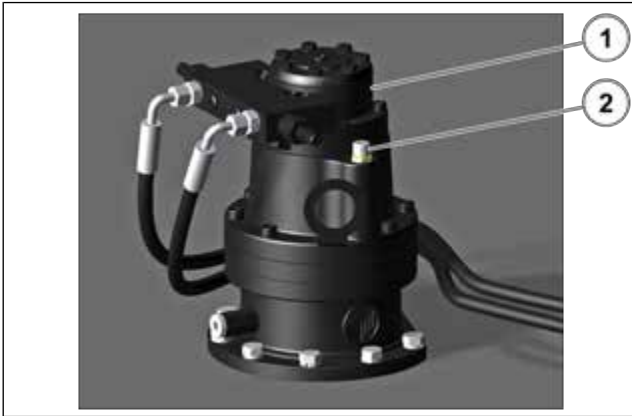
Figure 107: Checking the oil level of the turntable rotation motor 1
