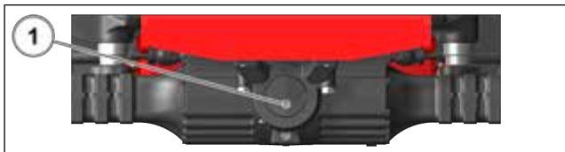
Figure 86: Checking the front axle differential for leaks
