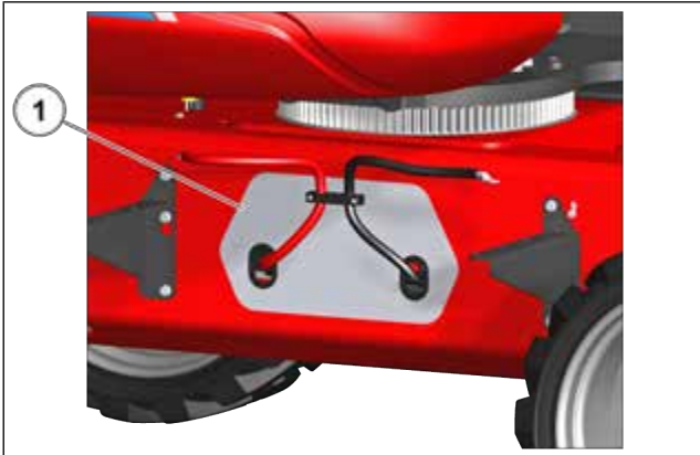
Figure 110: Checking the cables and the 12 V electrical connections 1
