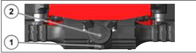
Figure 145: Replacing the front axle differential oil
