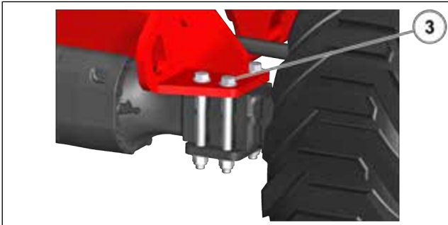
Figure 98: Checking axle tightness 4
