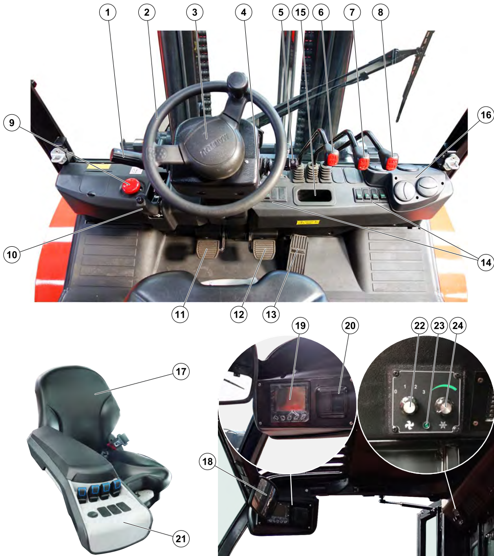
Figure 13: Driver's cab components location – MI 50L→100 D D ST5 S1
