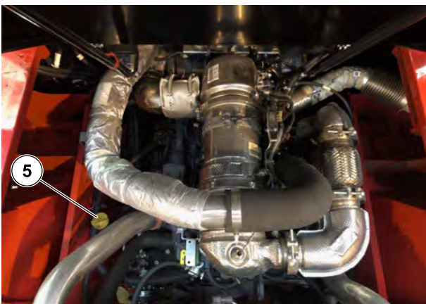
Figure 49: Filler plug - MI 80→100 D D ST5 S1
