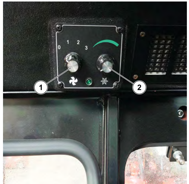
Figure 26: Air conditioning controls
