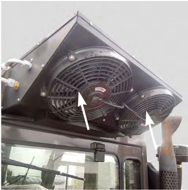
Figure 61: Direction of the compressed air flow through the air conditioning condenser core
