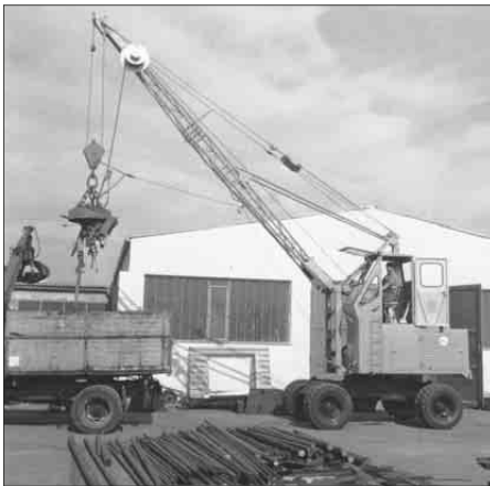
1962: Rope-driven S833 with elevated operator cab
