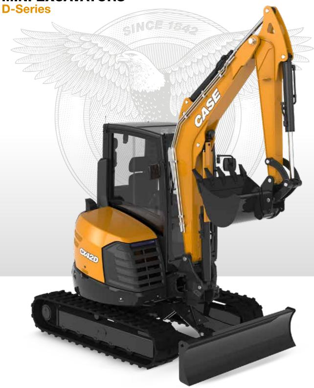
Engine D1803-CR-T Engine power 32.3 kW - 43.9 hp Operating weight 4200 kg
