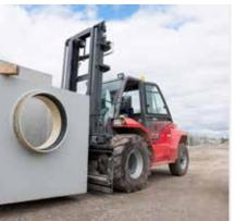
Thanks to its mechanical linkage, with an engine located at the rear of the machine, the MH is an exceptionally compact machine (less than 2m in height), boosting a capacity (2 to 2.5 tonnes). MHs feature a Kubota engine with 48.6 Kw (Stage 3B) or 36 kW (Stage 3A) power.
